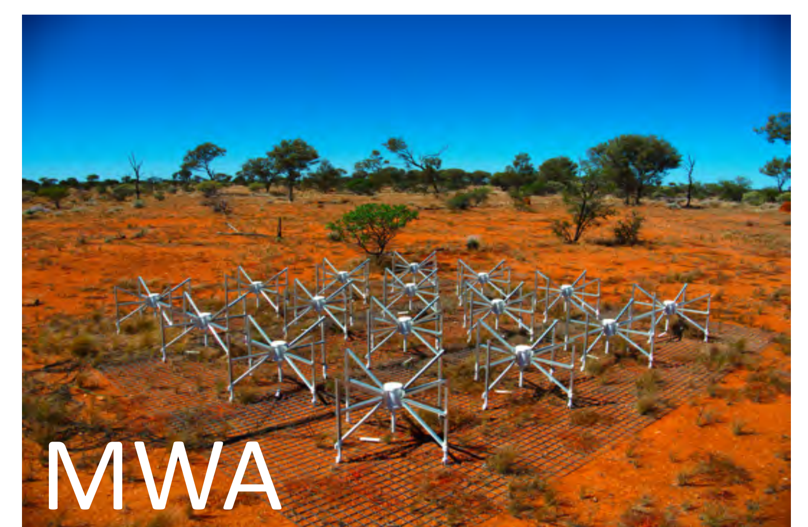
Figure 3: The Murchison Widefield Array is located in Western Australia and observes at 70 – 300MHz. It offers 3072 frequency channels with a resolution of 10kHz.
