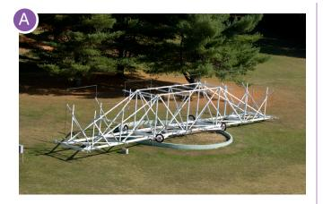
The Jansky Antenna (A) is an exact replica of the antenna used by Karl Jansky in the early 1930s. With it, he found three sources of radio static: two were caused by thunderstorms, but he concluded that the third was coming from the Milky Way! After hearing of Jansky's cosmic static, radio engineer Grote Reber was determined
