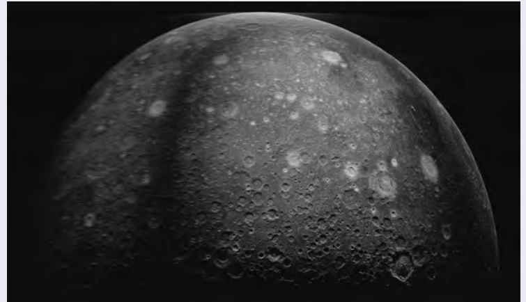
In this image, north is up and the bright crater at the upper right is Theophilus. The dark ring in the image is due to the pattern formed by the transmitting and receiving antennas. (AUI, GBO)
